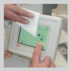
Simple programming of the seam segment for different contours (e.g. collars) with the use of the keyboard/display
